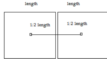
Fig 5 The spacing between two adjacent pixel centers (Pixel Spacing) is equal to the pixel length
