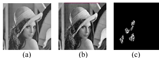
Fig. 6 (a) Original image (b) Watermarked image (c) Difference which shows those areas which are tampered
