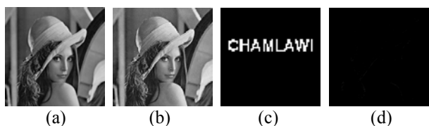
Fig. 4 (a) The watermarked image (b) the recovered Image (c) The extracted binary signature (d) Difference in original and extracted binary signature
