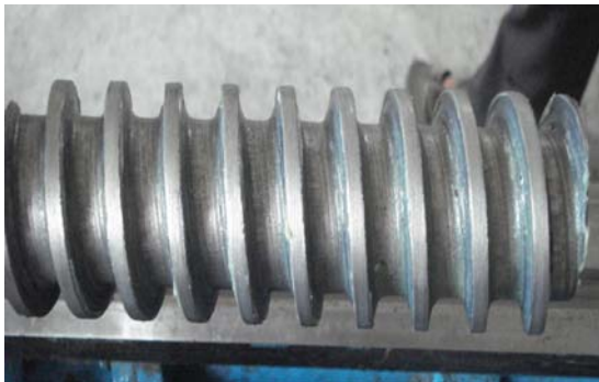
Fig. 2 Mandrel having the profile of the spring
