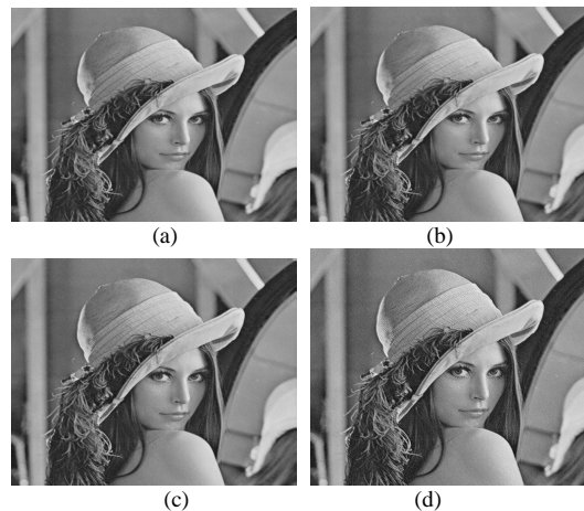
Fig. 2 The stego-images of "Lena" at the different pure payload. (a) 41.77 dB embedded with 0.5 bpp, (b) 37.92 dB embedded with 0.70 bpp, (c) 32.61 dB embedded with 1.0 bpp, and (d) 25.22 dB embedded with 1.50 bpp
