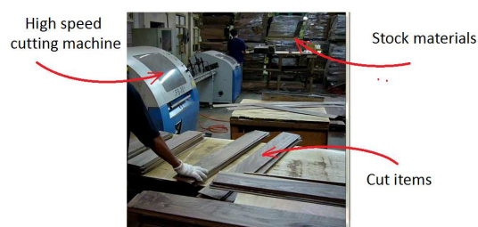
Fig. 1 A production line for high-speed floorboard cutting
