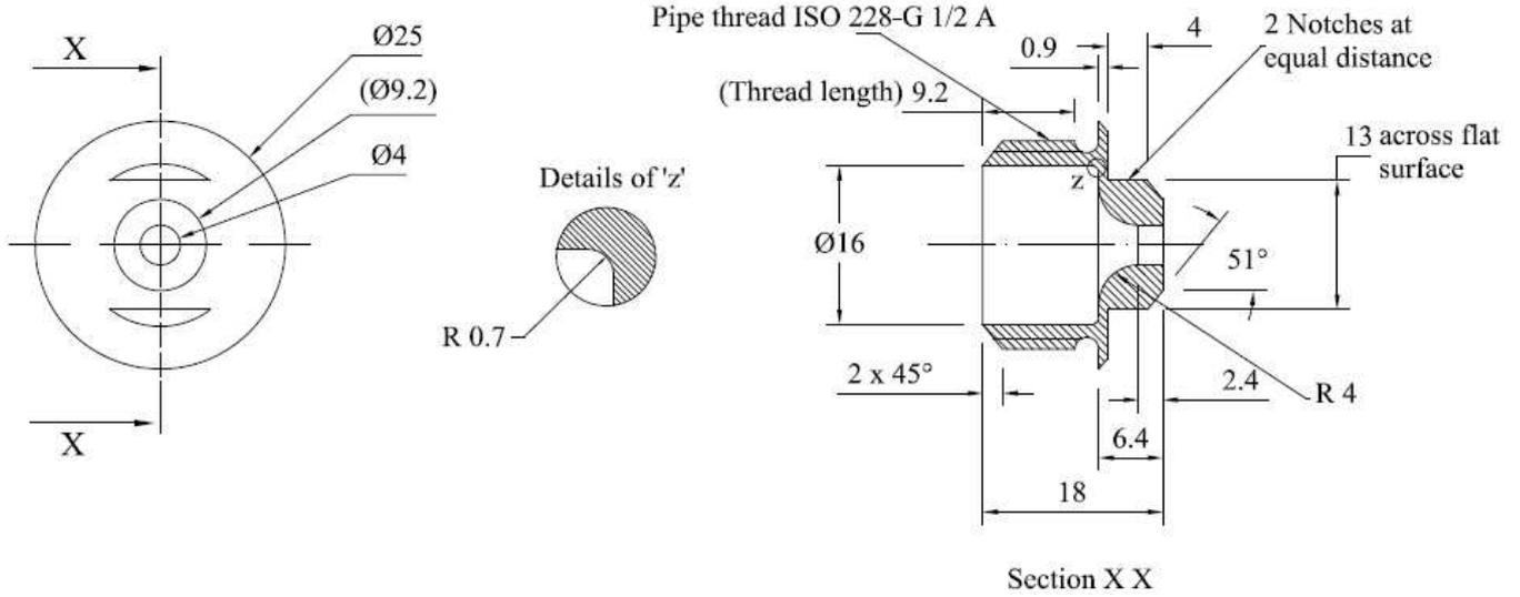
Fig. 2 (a) Sectional view of primary device with circular profile
