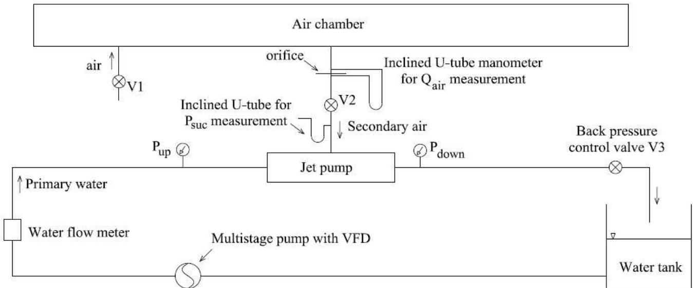
Fig. 3 Schematic arrangement of two phase flow jet pump test set up
