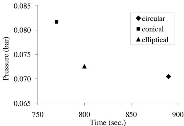
Fig. 13  $t_{critical}$  &  $P_{critical}$  with different profiles
