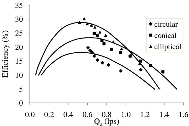
Fig. 8 Performance comparison at  $S = 32$  mm &  $Q_w = 0.444$  lps
