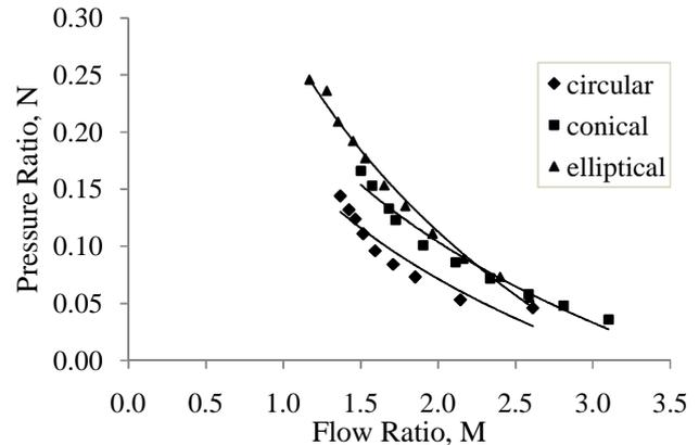
Fig. 6 Dimensionless plot showing the comparison at  $S = 32 \text{ mm}$  &  $Q_w = 0.444 \text{ lps}$
