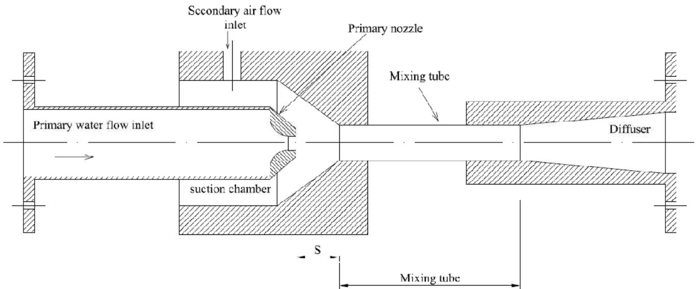
Fig. 1 Cross section of jet pump along with mixing tube and diffuser
