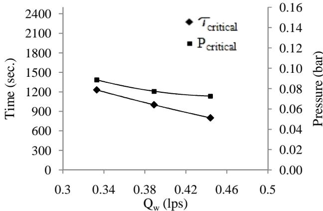
Fig. 11 Critical points for various  $Q_w$  with elliptical profiled nozzle at 32 mm of nozzle spacing
