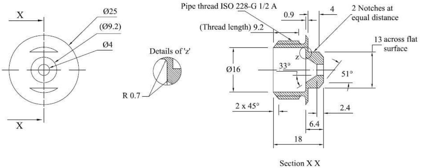
Fig. 2 (b) Sectional view of primary device with conical profile
