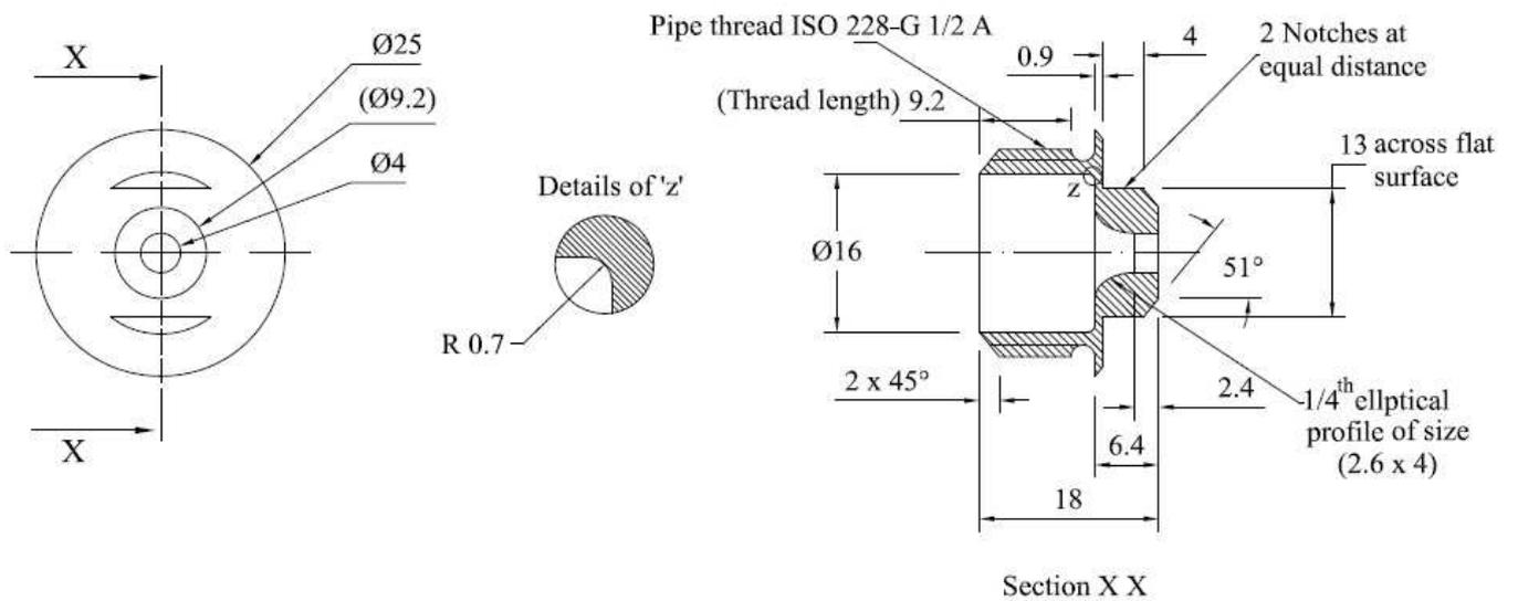
Fig. 2 (c) Sectional view of primary device with elliptical profile
