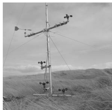
Fig. 3 Mast cup anemometers were installed at 0.2 m, 0.5 m, 1 m, 2 m and 5 m heights
