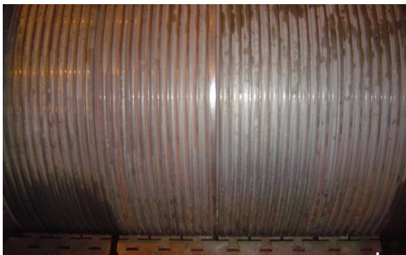
Fig. 1 Effects of rubbing on rotor surface
