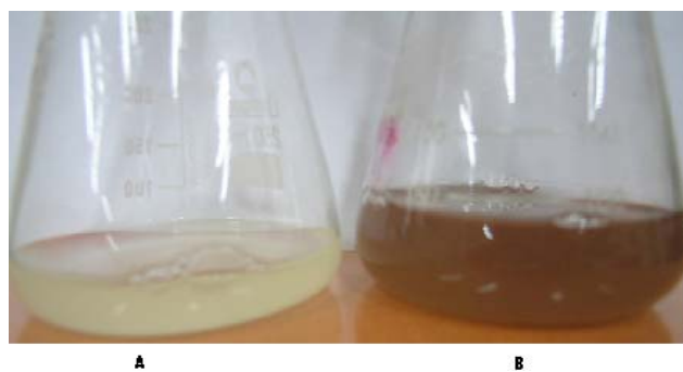
Fig. 1 Fungal filtrate of Aspergillus species in conical flask (A) control flask (B) after 24 hours reaction with silver nitrate
