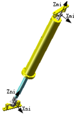
Fig.3 One Leg of the 6-DOF parallel robot
