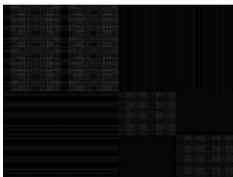
FIGURE 12. DIFFERENCE IMAGE BETWEEN NYQUIST PATTERN AND JPEG COMPRESSED IMAGE. PSNR RATIO IS 29,3 DB
