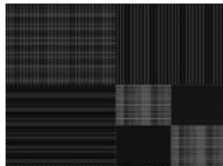
FIGURE 11. DIFFERENCE IMAGE BETWEEN WAVECODEC AND ORIGINAL NYQUIST PATTERN. PSNR RATIO IS 25,9 DB
