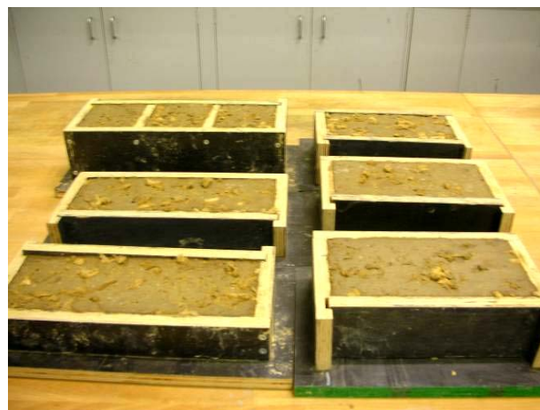
Fig. 2 Compacted bricks, beams and cubes (soil-CBs mix)
