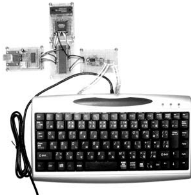
Fig. 2. Prototype of keystroke pressure measurement system with a keyboard.
