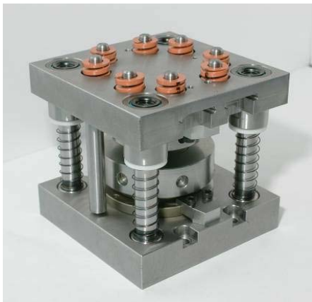
Fig. 7 Die set and spring structure
