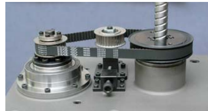
(a) Pulley driven structure
