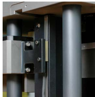
Fig. 5 The linear displacement sensor that have a resolution of 0.1um
