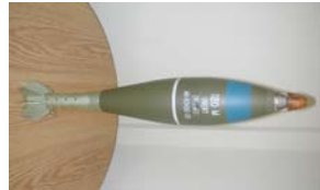
Fig. 2 The non-rolling finned 120 mm HE mortar projectile
