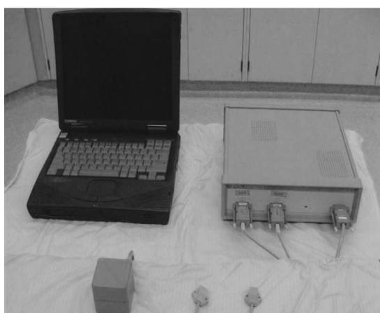
Fig. 2 Hand-motion analysis was recorded using Imperial College surgical assessment device (ICSAD) [9]
