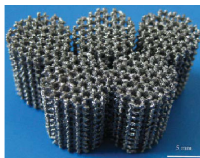
Fig. 10 The EBM fabricated Ti-6Al-4V implants with honeycomb structure [95].
