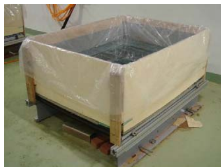
Fig. 4 2400Pa water pressure applied on the module
