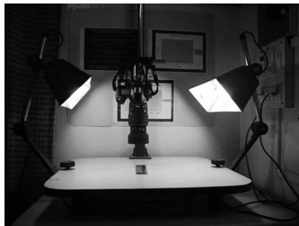
Fig. 4 Experimental set-up for Image Acquisition
