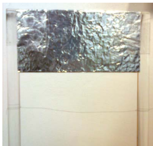
Fig. 1 A detail of the asymmetrical capacitor
