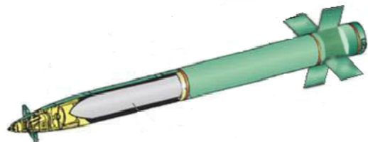
Fig. 1 Canard controlled 122mm rocket with straight tail fins
