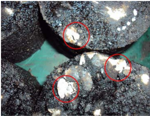
Fig. 4 Broken aggregates during compaction
