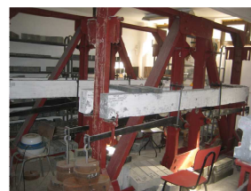
Fig. 3 Aspects regarding beams subjected to long-term loading
