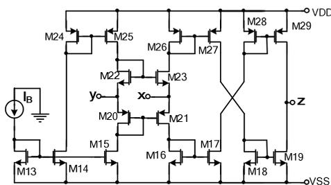
Fig. 5 Internal construction of CCCII
