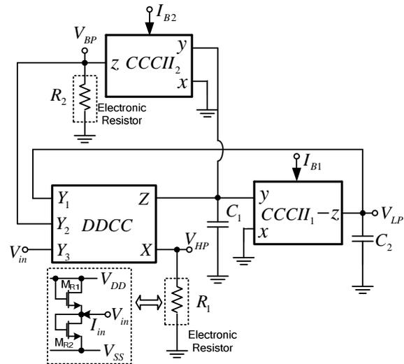
Fig. 3 Proposed voltage-mode universal filter
