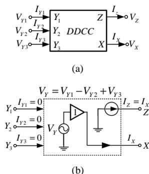
Fig. 1 DDCC (a) Symbol (b) Equivalent circuit
