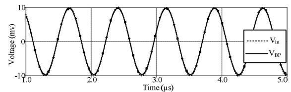
Fig. 8 Transient response of band-pass function
