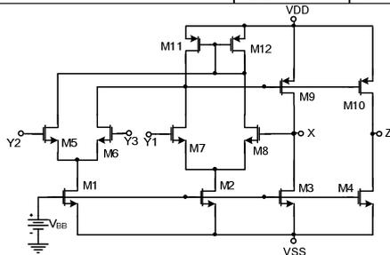
Fig. 4 Internal construction of DDCC
