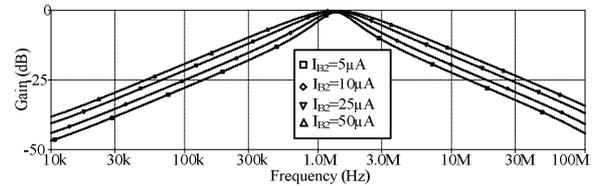
Fig. 7 Band-pass responses for different values of  $I_{B2}$
