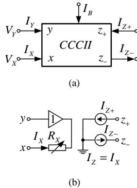
Fig. 2 CCCII (a) Symbol (b) Equivalent circuit
