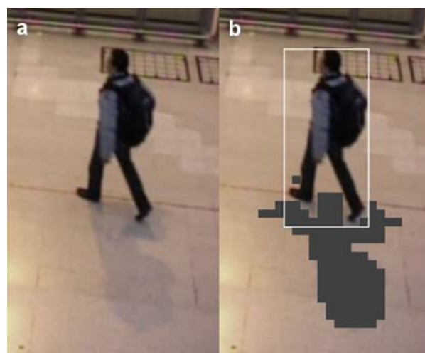
Fig. 3 Shadow detection and cancellation. a, original image. b, detected shadow (gray blocks) and blob bounding box (white)
