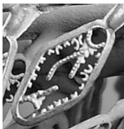
Fig. 11 The incomplete filling filigrees were cast at the T-casting 1293 K and T-flask 933 K
