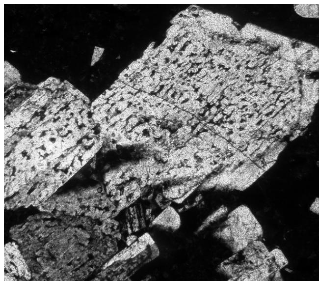
Fig. 4 Sieve textured plagioclase phenocrystals in DVS lavas
