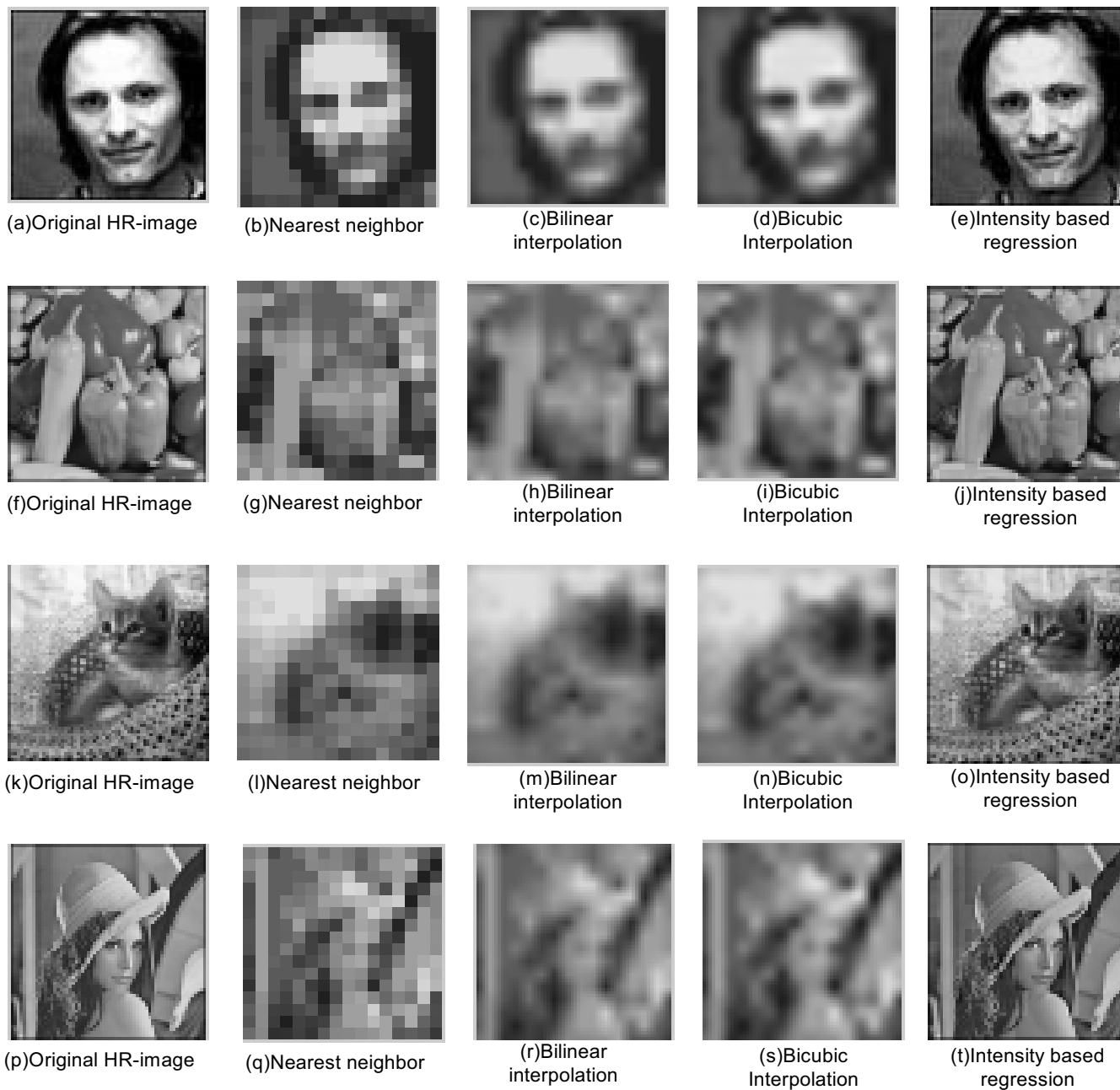
FIG.3.Comparison of 64x64 images, Fig 3(a)-3(d) Results of experiments conducted on the face image, Fig 3(f)-3(j) Results of experiments conducted on the peppers image, Fig 3(k)-3(o) Results of experiments conducted on the cat image, Fig 3(p)-3(t) Results of experiments conducted on the Lena image.
