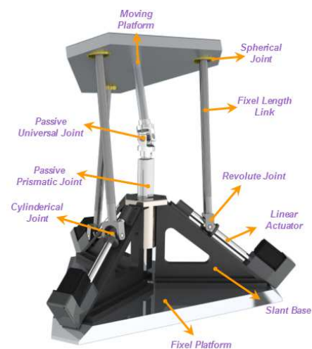
Fig. 1 CAD model of 3-CRS/PU parallel manipulator
