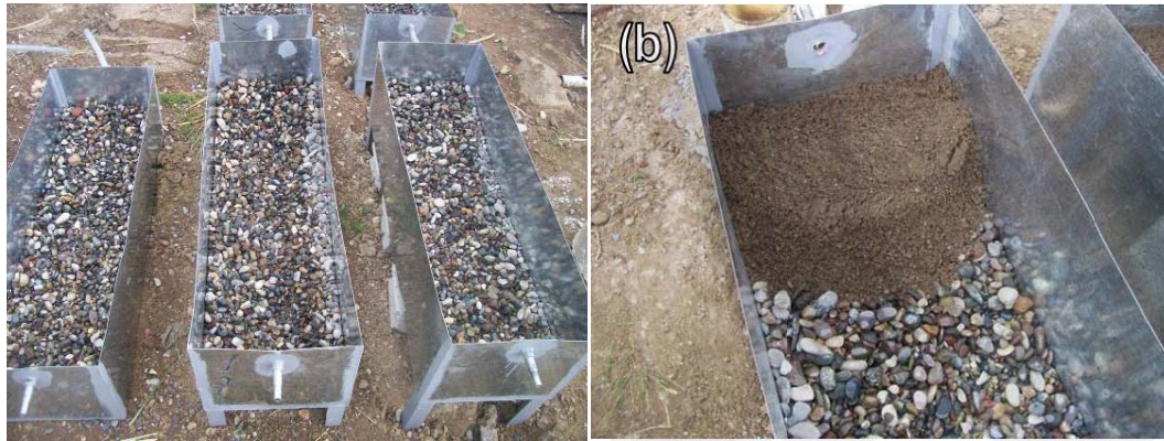
Plates 5 and 6 Microcosm construction wetlands preparation stages and design.
