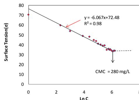
Fig. 2 Surface tension reduction with greywater concentration
