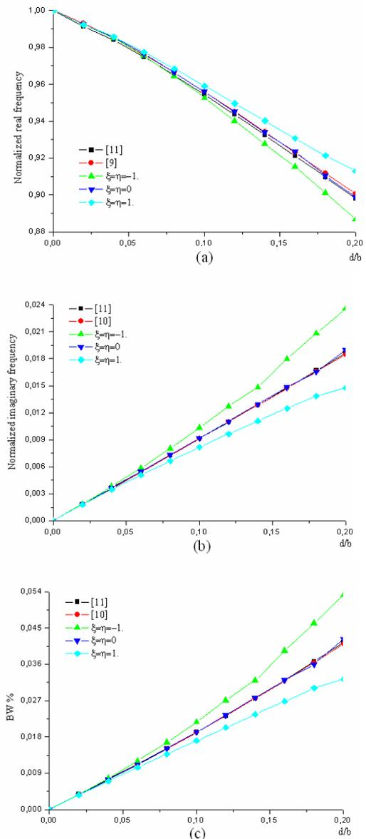
Fig. 2 Normalized resonant frequency,  $a=1.5\text{cm}$ ,  $b=1\text{cm}$ ,  $\varepsilon_z=7$  (a) real part (b) imaginary part (c) Half-power bandwidth
