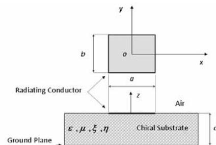
Fig. 1 Rectangular Microstrip Patch Antenna with Chiral substrate
