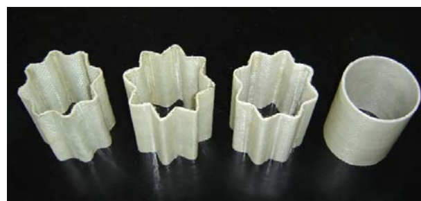
Fig. 1 Tested specimens (Right to left CCT, RCCT, TRCT, TZCT)
