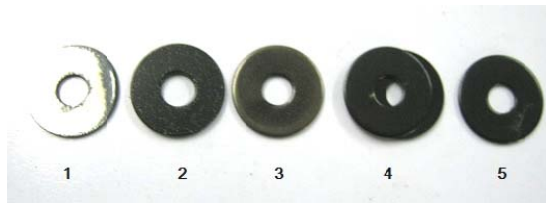
Fig. 1 Types of electrocoating defects
