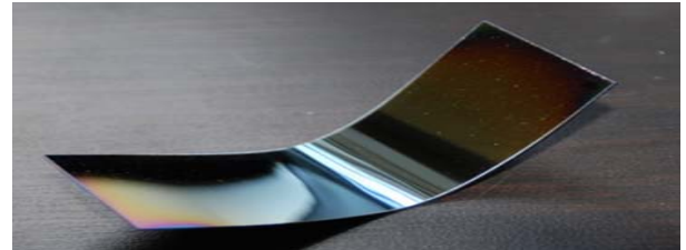
Fig. 9 Si foil of radius 252 mm shaped by hot plastic deformation
