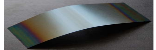
Fig. 10 Si foil of radius 398 mm shaped by hot plastic deformation
