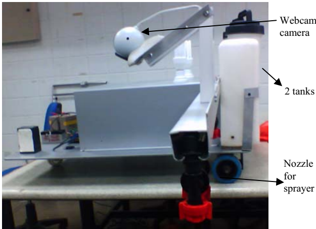
Fig. 3 The sprayer structure of the automated weeding strategy
