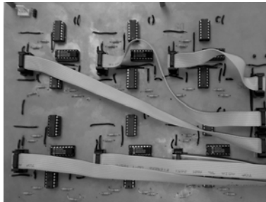
Fig. 2 Signal Conditioning Circuit
