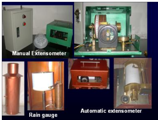
Fig. 5 Early warning system equipments consist of a) manual extensometer with the control panel and syringe and b) rain-gauge [4].
