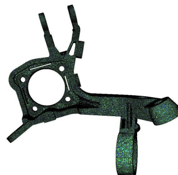
Fig. 15. Stub axle [14]. Colormap according to the quality of the triangles
