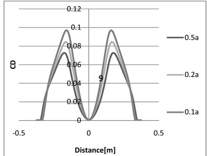
Fig. 18 Dimensionless shear stress CD, for three different curved profiles – local distribution
