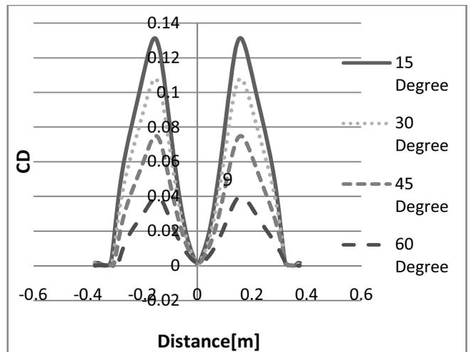
Fig. 14 Dimensionless shear stress CD, for four different nozzle angle – local distribution
