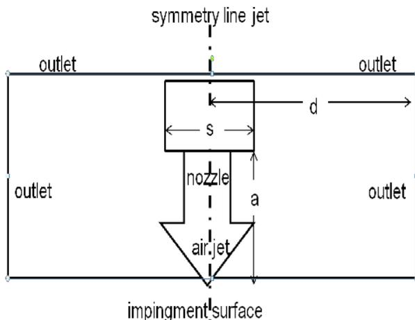
Fig. 2 Model Geometry
