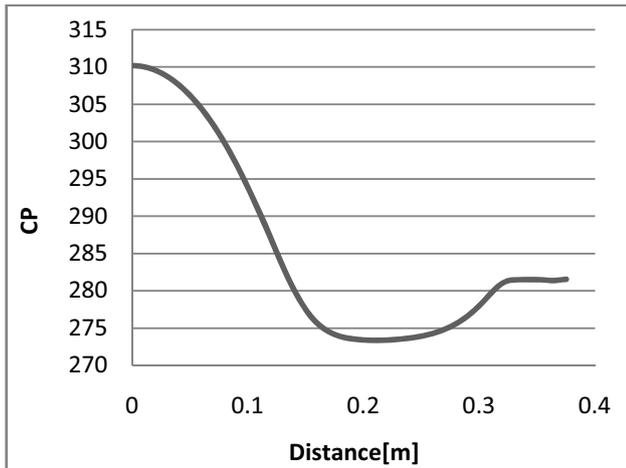
Fig. 5 Dimensionless normal pressure CP – local distribution
