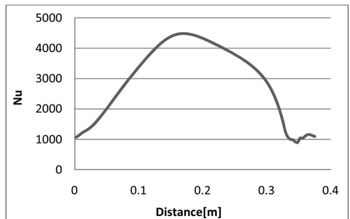
Fig. 4 Dimensionless heat transfer coefficient Nu – local variation
