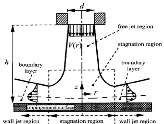
Fig. 1 Three different region of flow in jet impingement on a wall, nozzle diameter  $d$  and distance  $h$  [9]
