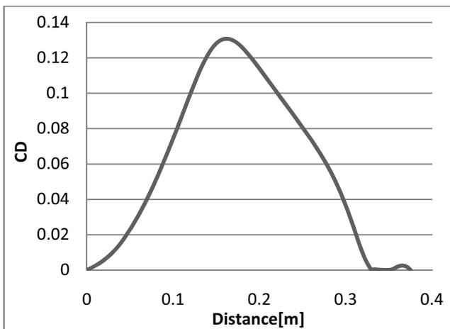
Fig. 6 Dimensionless shear stress CD – local distribution
