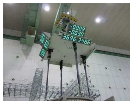
Fig. 2 Physical appearance of the hoist device
