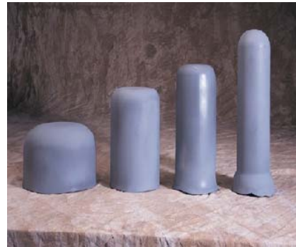
Fig. 3 Specimen that have been successfully drawn
