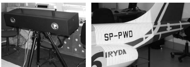
Fig. 3 Three-dimensional structured light scanner; example of the measuring process (projection of the raster)
