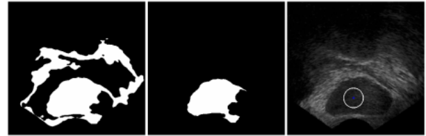
Fig. 7 Binarization the image(left), select the most area region(middle), inside point finding(right)
