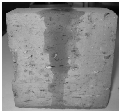
Fig. 1 Ceramic brick filled by siloxane injection
