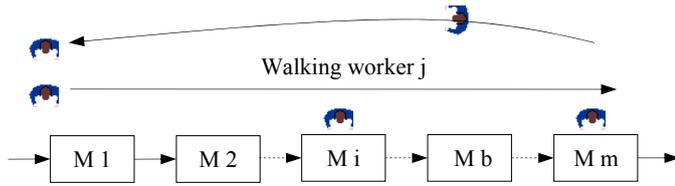
Fig. 1 The linear walking worker assembly line
