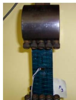
Fig. 1 Test set up of CFRP
