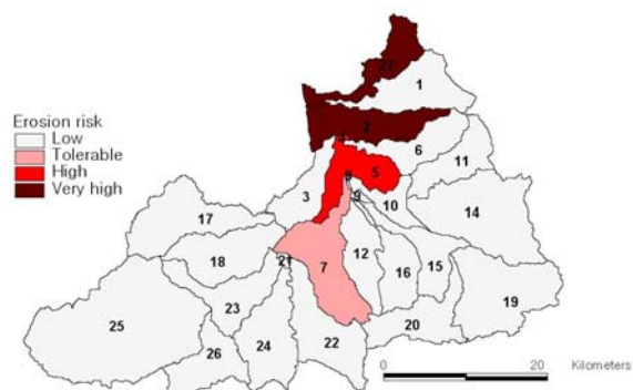
Fig. 2 Spatial distribution of sediment yield predicted by SWAT in the Sarrath catchment
