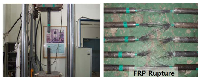
Fig. 5 View of tensile test and failure pattern
