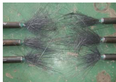
Fig. 9 Failure pattern of 3-multi CFRP tendon
