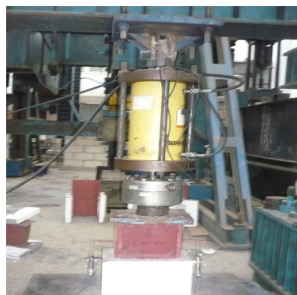
Fig. 3 Push-out specimen under testing
